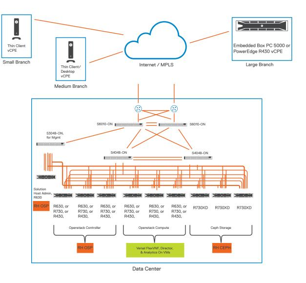
Figure 1: Network diagram for Dell EMC, Red Hat and Versa solution
