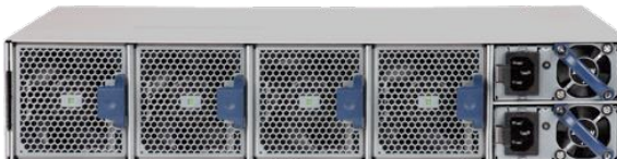
Arista 7260X 2RU Rear View: Rear to Front airflow (blue)
